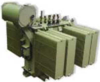
Converter transformer, 19400 kVA, three-windings supply of LCI-drives.
